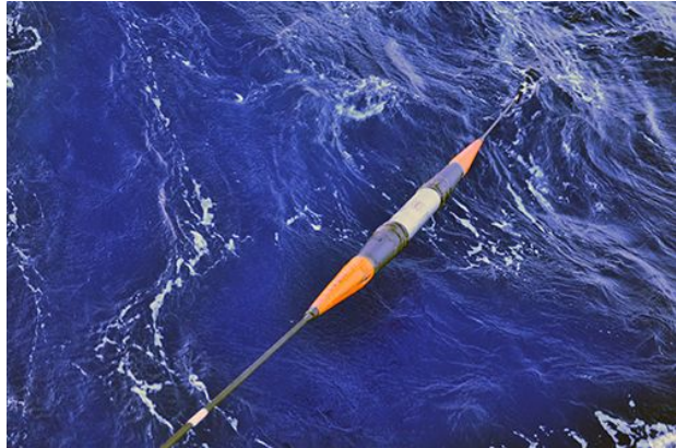
Fig. 3 (a) Crew members load an optical repeater (in wooden cradle) on the deck of Orange Marine's Pierre de Fermat cable ship near Brest, France, during the deployment of an Xtera submarine telecommunications cable system. (b) An optical repeater slips beneath the waves as the cable it is attached to is deployed along the ocean floor. Credit for both photos: Bertrand Clesca, Xtera.
