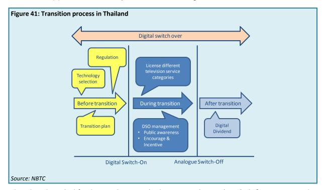
The selected standard for the Digital Terrestrial Television Broadcasting (DTTB) platform is DVB-T2. The DTTB platform includes five multiplexes (to be extended later to six) and these networks carry the six incumbent television services and hence the six incumbent television services are simulcasted in the DTTB coverage areas. In the fully deployed stage the DTTB network will cover 95 per cent of the households in Thailand.
