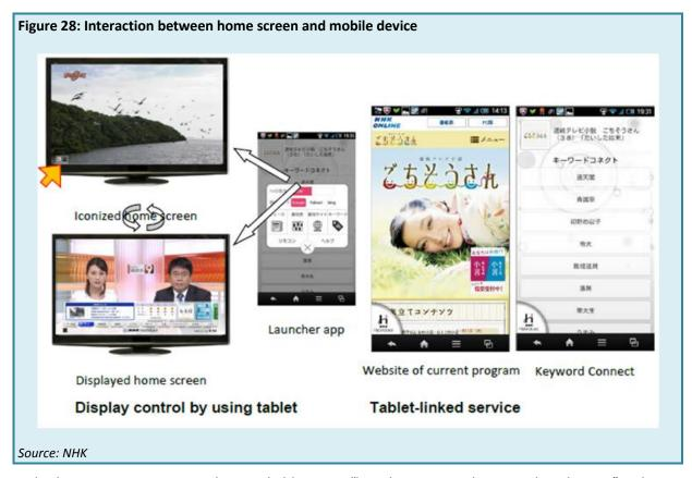
Hybridcast services are currently provided by using "broadcast-oriented managed application". When a service is about to start, a broadcaster transmits a control signal to for example terrestrial television receivers to launch an application automatically. The broadcaster creates an application and distributes it to each viewer, so a viewer can feel safe to use it.
