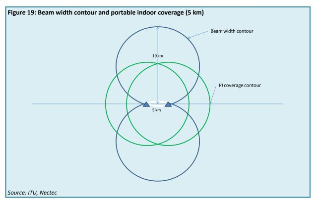
Figure 19 shows that in significant areas around the transmitter sites viewers will have problems receiving all services as the beam width contour is much larger than the overlapping portable indoor coverage area. The beam width contour will be smaller when the sites are located closer together. When the sites are two kilometres apart the beam width contour will fall with the overlapping portable indoor coverage area and hence the viewers will have no problem receiving all services.
