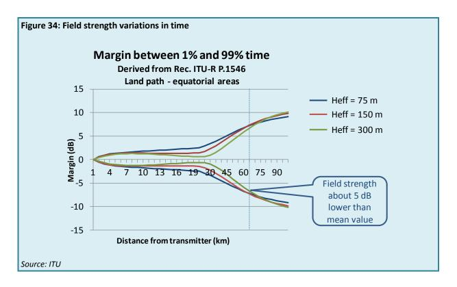
Figure 34 shows that up to about 25 km from the transmitter the time variation is relative small. At larger distances the variation increases and is about 10 dB higher than the mean value for 1 per cent of time and about 10 dB lower for 99 per cent of time<sup>61</sup>. The frequency planner is faced here with the question of what an acceptable variation is.
