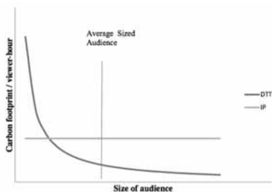
Figure 13: The relationship between carbon footprint per viewer-hour for DTT and video-on-demand and the size of the audience.
