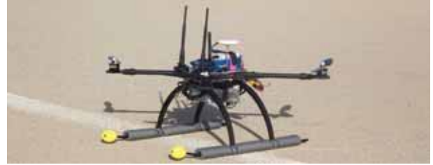
Figure 2. Drone used in the experimental aerial WiFi network.
