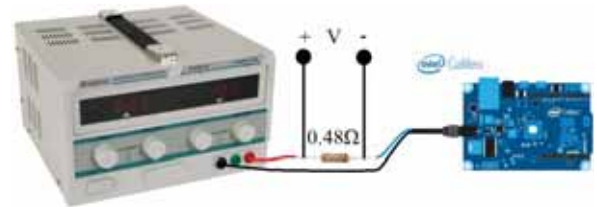
Figure 3. Experimental setup for current consumption measurements.
